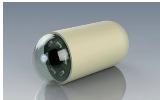
Figure 1: Depiction of a generic capsule endoscope [5].
