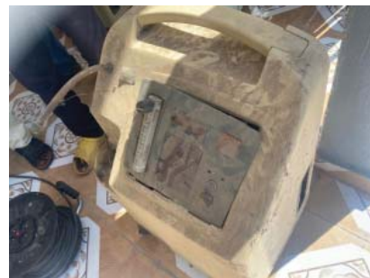
Figure 1: Illustration of the condition of a poorly maintained oxygen concentrator as found in some hospitals.
